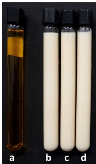
Figure 1 (a) Salmon fish oil, (b) Liposome made from phospholipid 2 % w/v, (c) Liposome made from phospholipid 3 % w/v, and (d) Liposome made from phospholipid 4 % w/v
