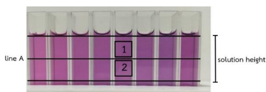
Figure 2 Position of photo analysis using Adobe Photoshop CS6 program applied for the proposed method.
