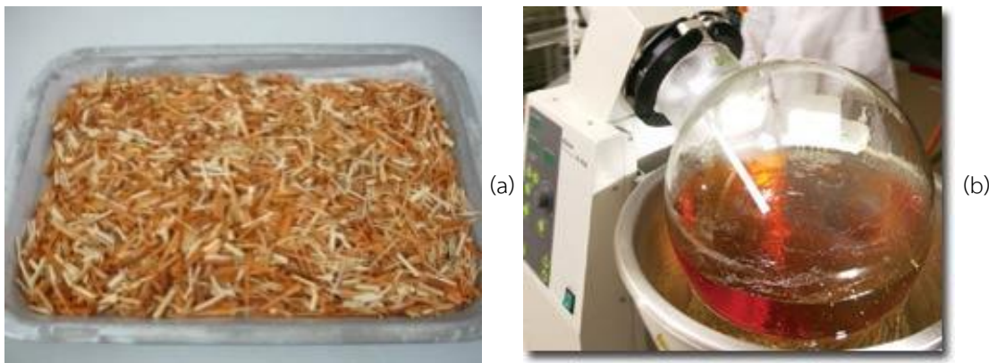
Figure 1 (a) Caesalpinia sappan heartwood was dried in hot air oven at 42 °C for 72 hours. (b) The methanolic extract of C. sappan was evaporated to dryness under vacuum using a rotary evaporator.
