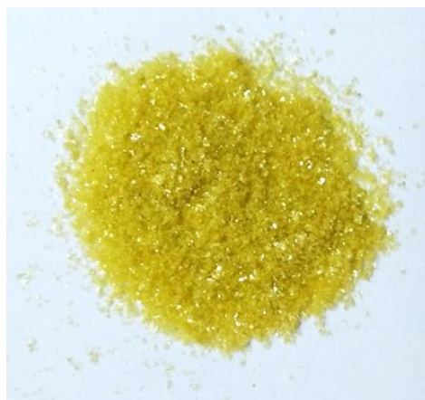
Figure 1 Yellow crystal of andrographolide isolated from Andrographis paniculata by liquid-liquid extraction with methanol: hexane (1 : 1) solvent
