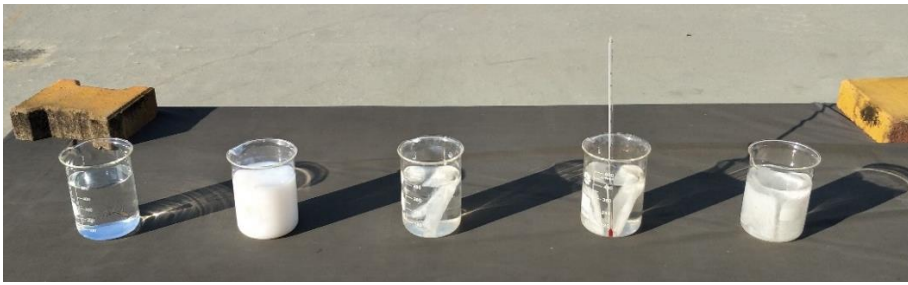
Figure 2 Experimental setups for control, Degussa P25 powder, and coated glass-fiber filters.
