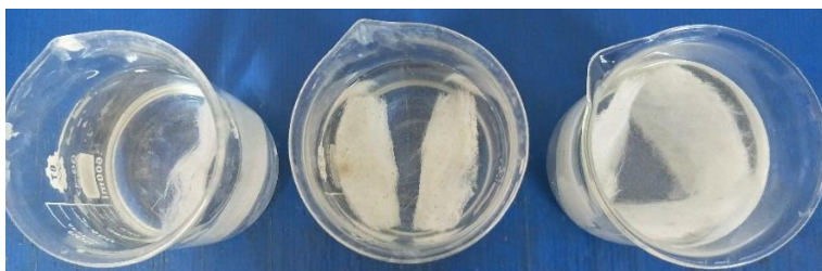
Figure 1 Positions of coated glass-fiber filters (1, 2, and 3 pieces) in beakers during photocatalysis.
