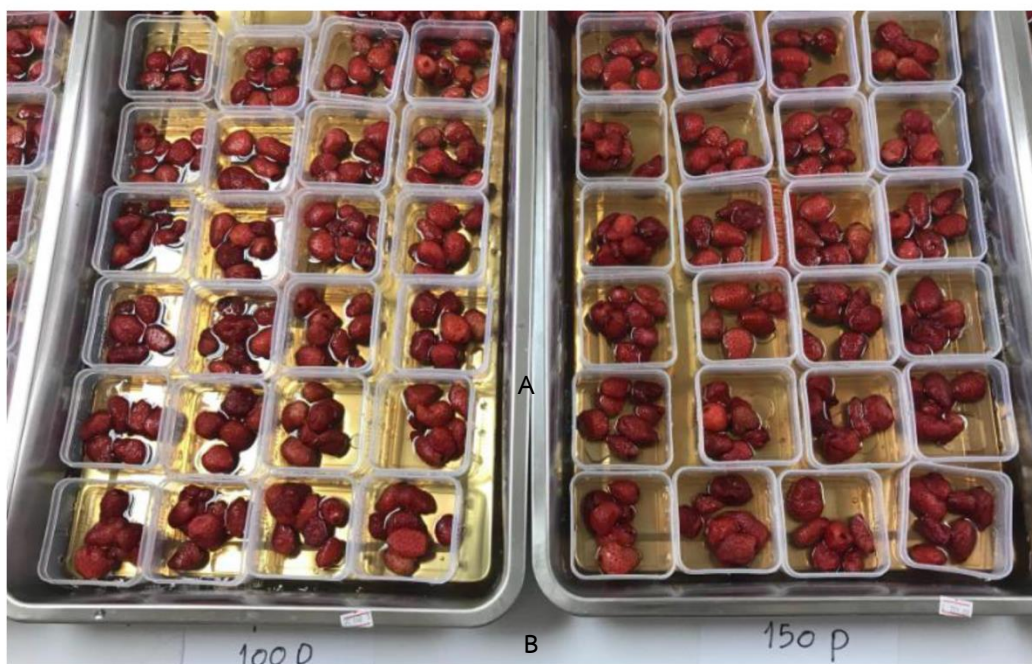
Figure 6 (a) Strawberry while pulsed electric field of 100 pulses and (b) Strawberry while pulsed electric field of 150 pulses
