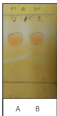
Figure 2 TLC of (A) standard berberine and (B) isolated compound from C. Fenestratum was performed along with on a silica gel plate using methanol:acetic acid: water (13: 0.7: 1). The orange spots were visualized by spraying with Dragendorff's reagent.
