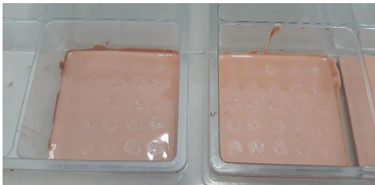
Figure 1 Condensation cure silicone rubber in square mold with small circle top coat
