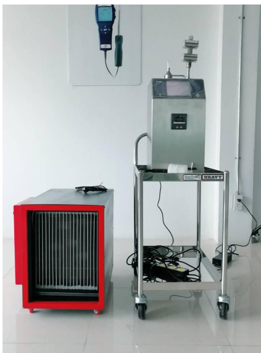
Figure 8 Experimental setup for evaluating the removal of bioaerosol of the developed air cleaner
