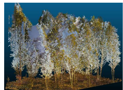
Figure 3 The results of converting multiple point cloud to a single point cloud
