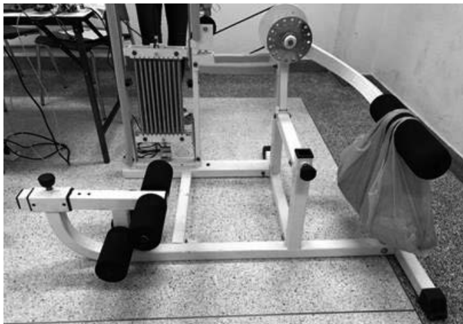
Figure 6 Testing the spring stiffness and load cell multiplier.
