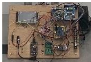
Figure 3 The command processing unit of the automated irrigation system with gravity pump.
