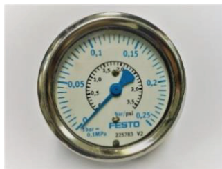
Figure 6 Pressure gauge (Festo) with resolution of +/- 0.005 bar.
