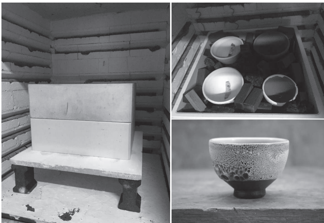
Figure 2 Firing set up in an electrical furnace of a closed box saggar refractory with charcoals placed on the bottom and fired samples.
