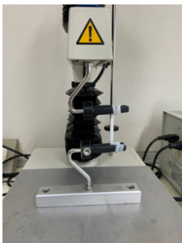
Figure 1 Textural measurement of cooked rice noodles using texture analyzer
