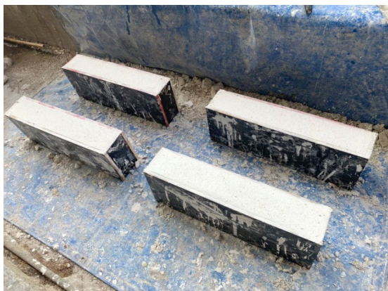
Figure 7 Sample of lightweight concrete blocks with hemp shiv
