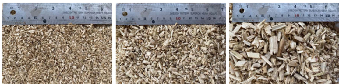
Figure 5 Ground Hemp Shiv size 6, 10 and 25 mm.
