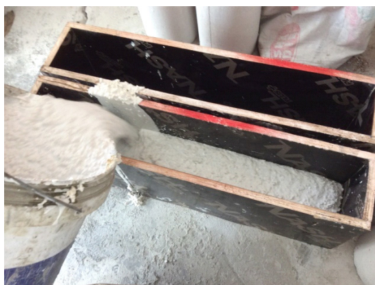
Figure 6 Mixed method of lightweight concrete blocks with hemp shiv
