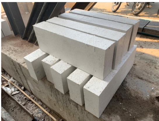
Figure 6 Mixed method of lightweight concrete blocks with hemp shiv
