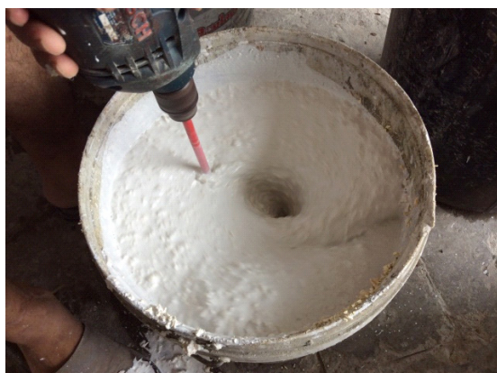
Figure 6 Mixed method of lightweight concrete blocks with hemp shiv
