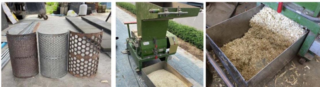
Figure 4 Hemp Shiv ground machine
