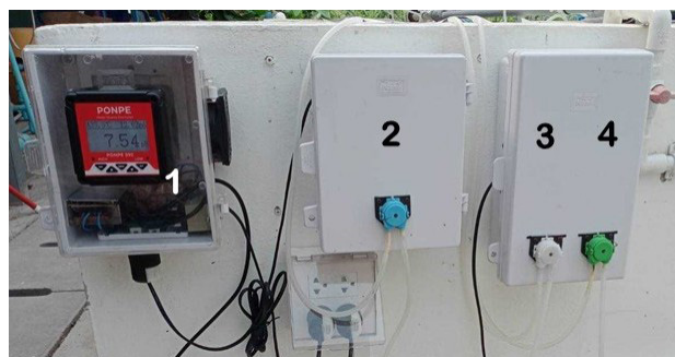
Figure 1 A pH measuring and controlling equipment set for macroalgae cultivation in a raceway pond
