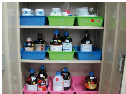
Figure 5 Chemical storage according to compatible groups and placement of chemicals on containment containers.
