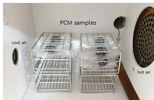
Figure 2 The photo shows a daily temperature cycle simulation test
